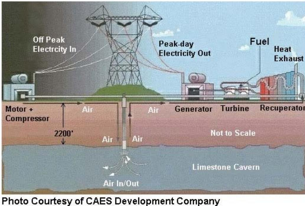
**Figure 5-11. Compressed Air Energy Storage**
