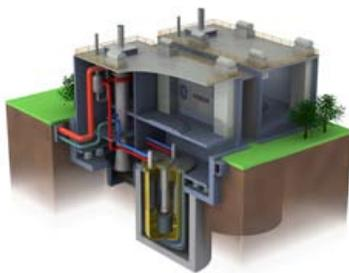
**311 MW(e) Power Reactor Innovative Small Module (PRISM), GE Hitachi Nuclear Energy** Liquid metal (sodium) cooled, underground containment on seismic isolators with a passive air cooling ultimate heat sink. Modular design with two reactor modules per power unit (turbine generator). NRC staff conducted pre-application review in early 1990s. 1 to 2-year refueling cycle.
