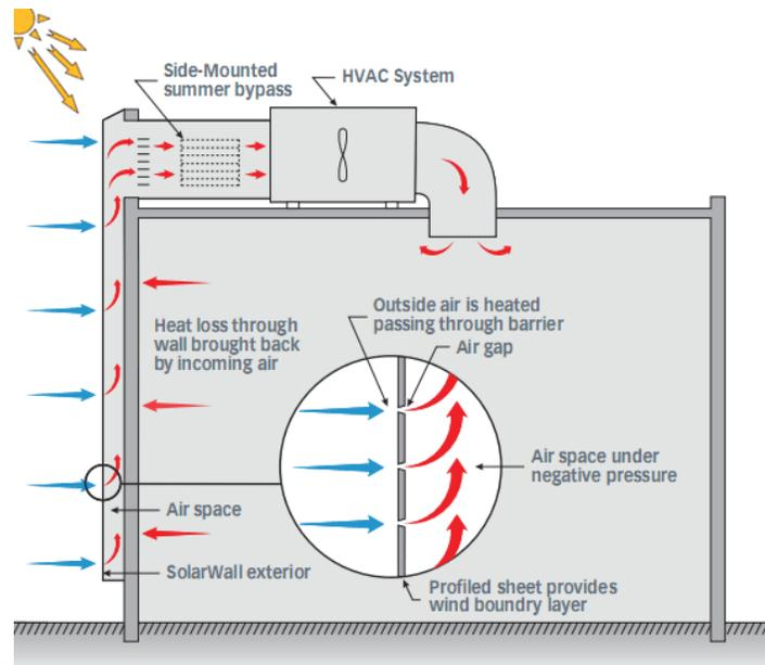
**Figure 5-6. Solar Ventilation Air Heating Diagram -SolarWall®**
