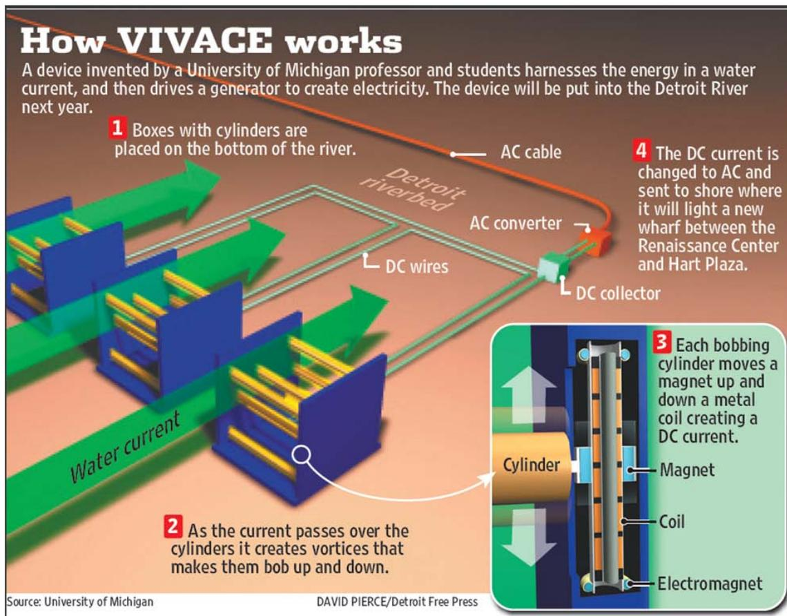
Figure 4-18. Vortex Induced Vibration Energy in Rivers
