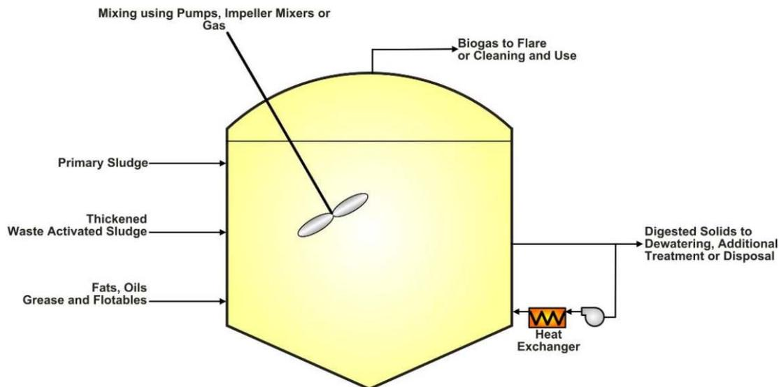
**Figure 4-3. Schematic of a Single Vessel Anaerobic Digester.**
