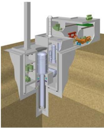
**10 MW(e) Super-safe, Small and Simple (4S), Toshiba Company** Small, sodium-cooled, underground reactor. Working with the city of Galena, AK as a potential COL partner. 30-year refueling cycle. Surface structure measures 72 feet by 52.5 feet, and 36 feet height. Ongoing pre-application meetings with NRC in FY2009. Ongoing pre-application meetings with the NRC, with Design Certification submittal in 2011. DC issued in 2014, and first 4S unit online in 2017.
