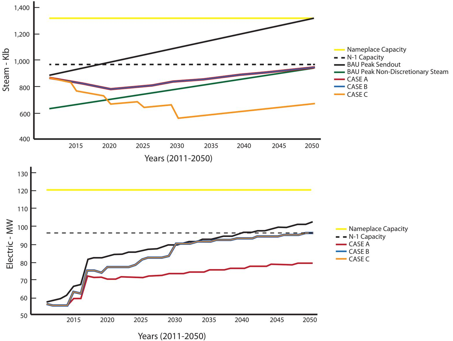
**FIGURE 9** In the steam and electrical capacity graphs, the dotted line represents the firm capacity, or the point in which additional steam or electricity will be needed. Scenario A (red) and B (blue) perform similarly, thus the lines overlap in the graphs
