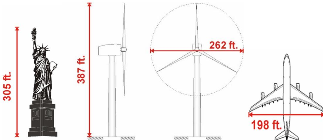
**Figure 4-13. 1.8 MW Wind Turbine Size Illustration**
