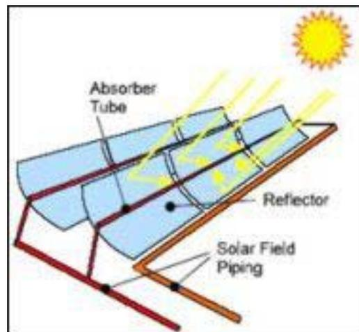
**Figure 4-11. Solar Thermal Power Trough Mirror Diagram**
