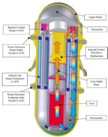
*335 MW(e) International Reactor Innovative and Secure (IRIS), Westinghouse Electric Company* Pressurized water reactor with reactor vessel, helical-coil steam generators, reactor coolant pumps, and pressurizer within a reactor vessel which is enclosed in a spherical steel containment vessel. 3 to 3.5-year refueling cycle.
