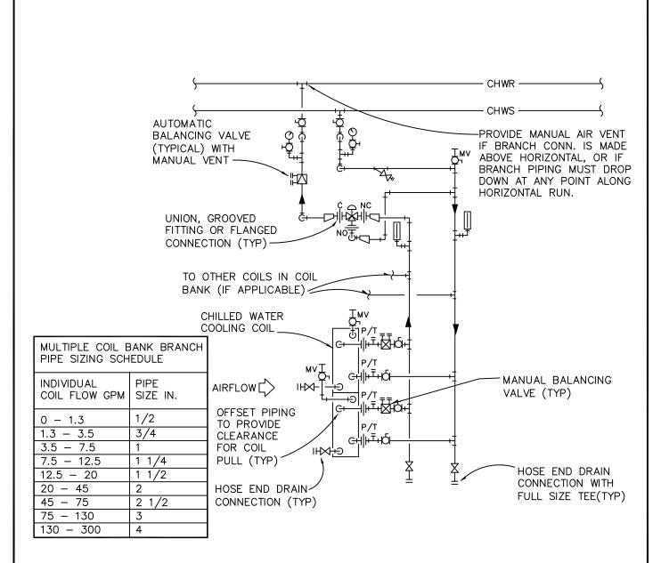
AHU CHILLED WATER COOLING COIL THREE-WAY CONTROL VALVE PIPING DIAGRAM WITH NO SCALE
