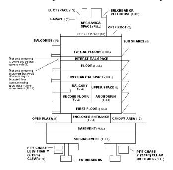
The STANDARD NET ASSIGNABLE AREAS are those portions of a building that are available for assignment as usable area or as rental area to an occupant.
