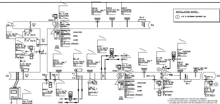
VARIABLE AIR VOLUME AHU WITH FLOWTRACKING AND VIFB STEAM HEAT CONTROL DIAGRAM
