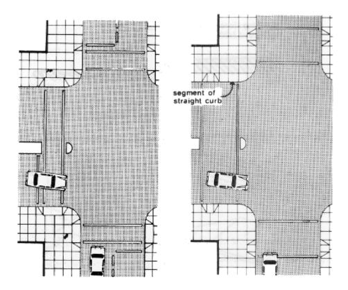
• The ramp slope is a ratio equal to the vertical rise (y) divided by the horizontal run (x). It is equal to the tangent of the angle that the plane of the ramp surface makes with a horizontal (level) plane. Transitions from ramps to walks, gutters, or streets shall be flush and free of abrupt changes. Maximum slopes of adjoining gutters, road surface immediately adjacent to the curb ramp, or accessible route shall not exceed 1:20
