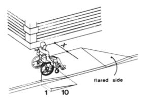
Note: if X is less than 48 in. then the slope of the flared side shall not exceed 1:12
