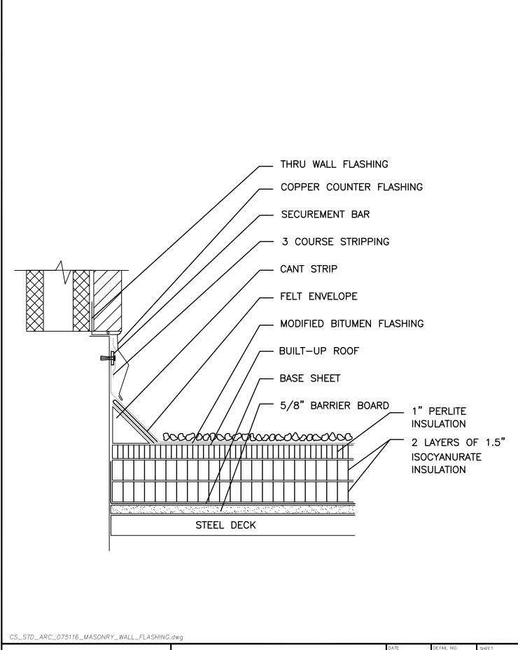
MICHIGAN STATE Infrastructure U N I V E R S I T Y Planning and Facilities MASONRY WALL FLASHING Typical Detail
