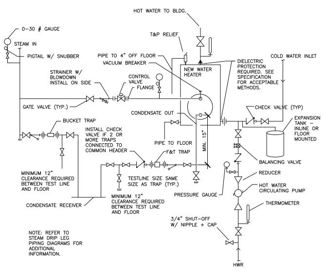
STEAM DOMESTIC WATER HEAT EXCHANGER PIPING DIAGRAM
