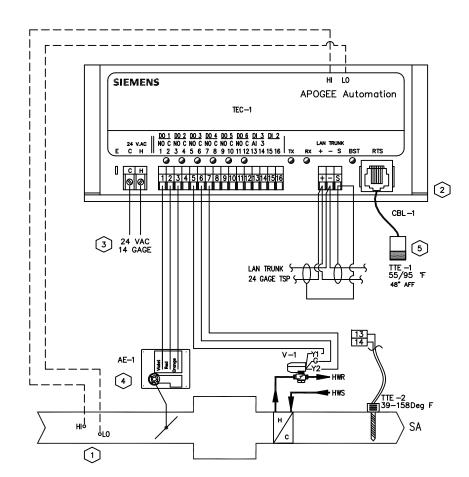
VAV WITH REHEAT CONTROL DIAGRAM
