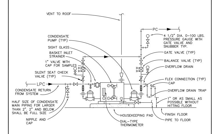
DUPLEX CONDENSATE RECEIVER PIPING DIAGRAM NO SCALE
