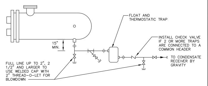
NOTE: FOR SYSTEMS WITH MULTIPLE TRAPS, INSTALL SHUT-OFF VALVE UPSTREAM OF STRAINER ON EACH BRANCH.
