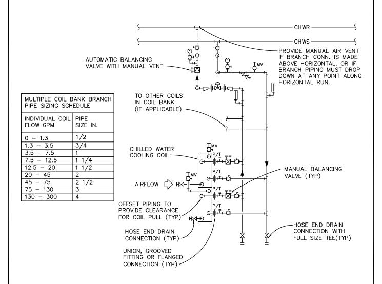
CHILLED WATER COOLING COIL WITH TWO-WAY
