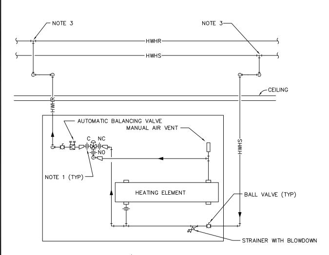
HWH CONVECTOR/CABINET UNIT HEATER PIPING DIAGRAM WITH THREE WAY CONTROL VALVE NO SCALE
