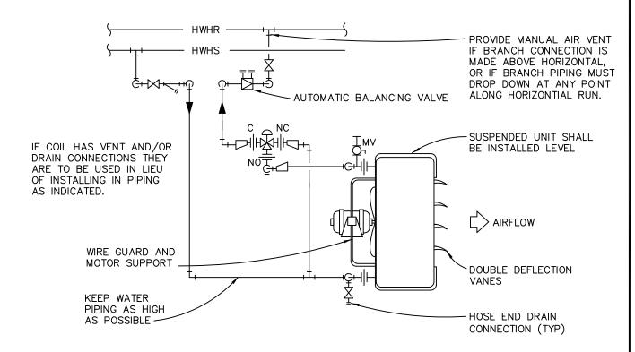
HOT WATER UNIT HEATER WITH THREE-WAY CONTROL VALVE PIPING DIAGRAM NO SCALE
