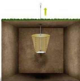
Soft Cohesive Soil (Based on Terzaghi's calculation)
